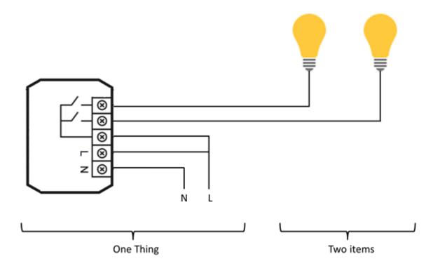
The actuator is the Thing. This might be installed in the electrical cabinet, it has a physical address and needs to be setup and configured in order to be used. The user is instead interested in the two lights, which are located at different locations in his home. These lights are the desired functionality, thus the Items and they are linked to the Channels of the actuator. A Link can be regarded like a physical wire in this example.
